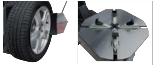
Bead breaker horizontal and vertically swiveling
